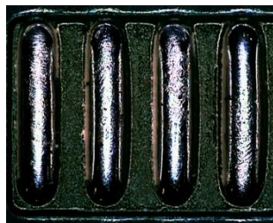
N 2 processing, excellent wetting and no flux residue
