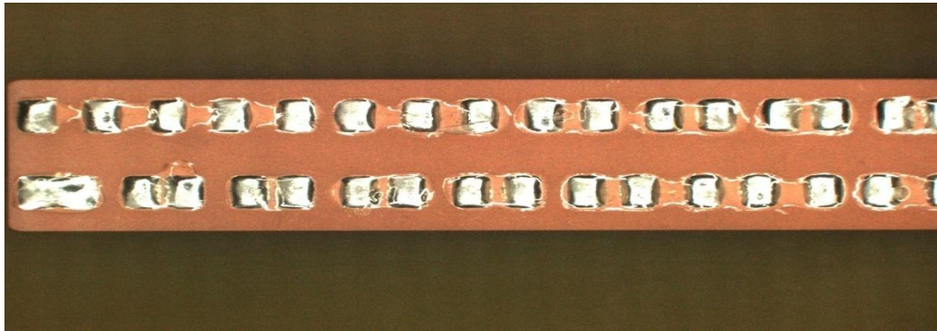
Figure 12. Poor wetting, with flux residue, high O 2 ppm levels > 5,000
