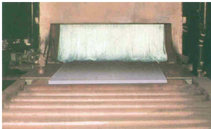
Figure3. A fiber cordage curtain at the exit end of furnace.
